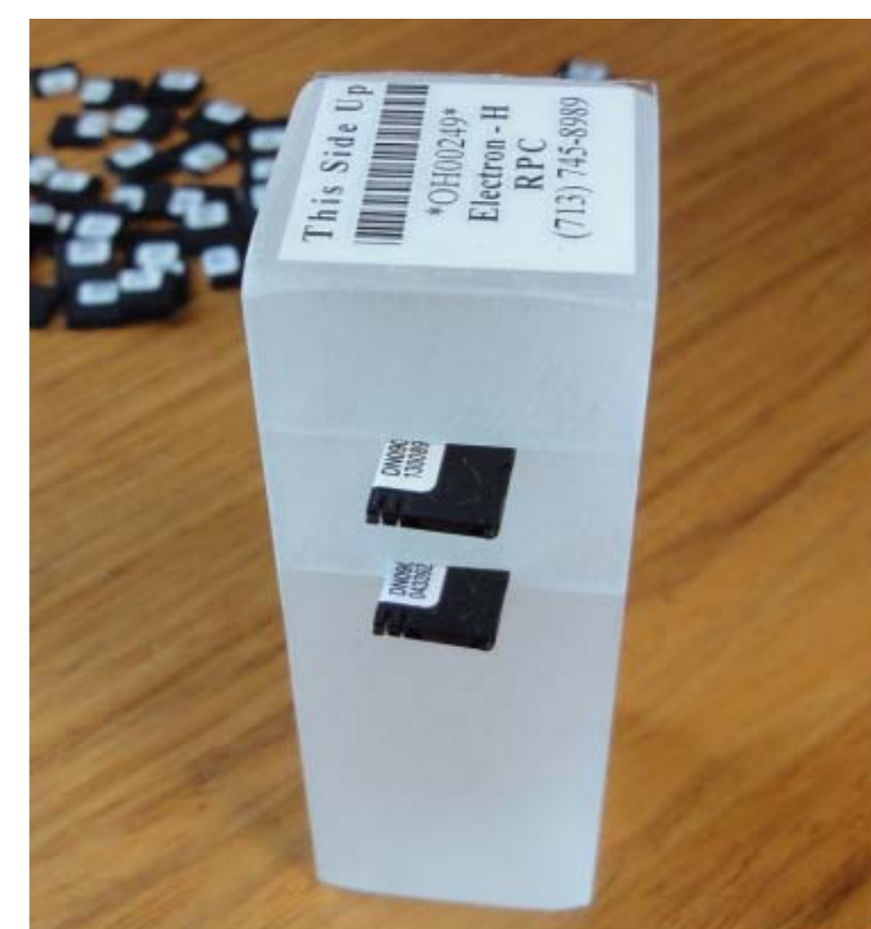
Standard RPC remote audit electron phantom. Two nanoDots™ are shown, at two different depths.
